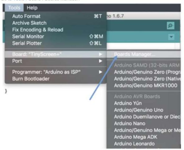
Select and install Arduino SAMD Boards (32 bits ARM Cortex-M0+) for Ardiuno/Genuino Zero/MKR 1000.
