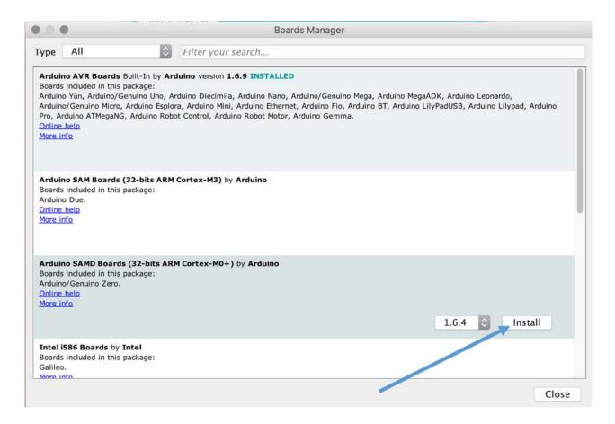
Then on the same Board Manager, scroll down to select and install TinyCircuits SAMD Boards.
